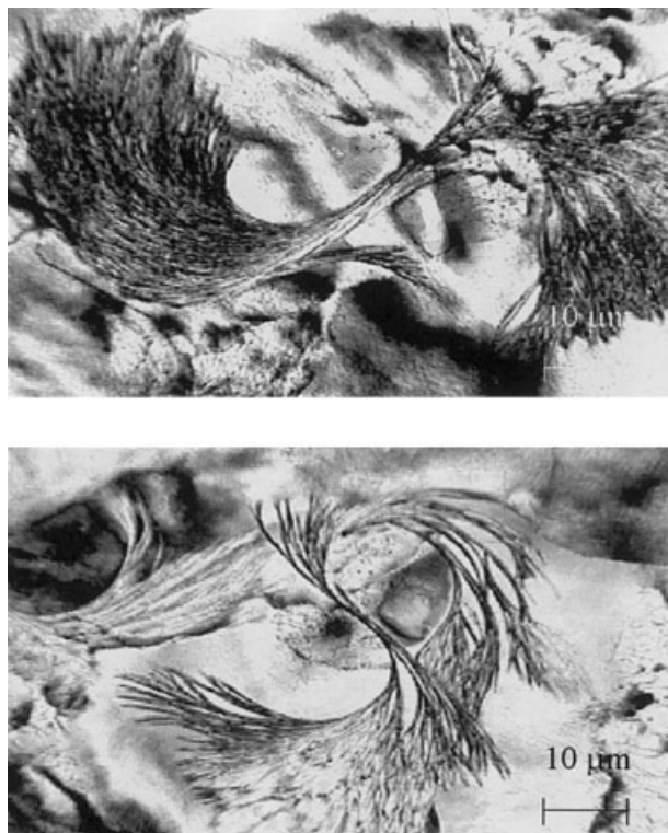
Figure 12 PLM micrographs of a PTHF/lauric acid blend.
